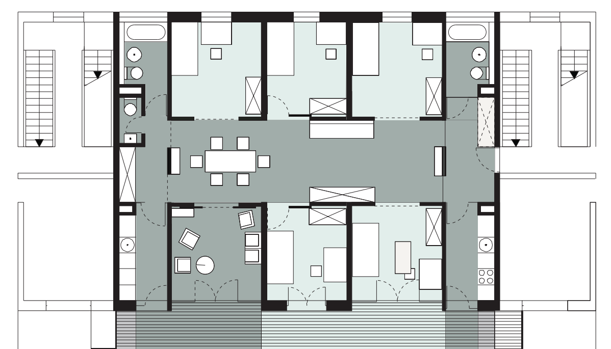
Additional space required via expansion; shared by 5 people with central dining/living and individual rooms around.
