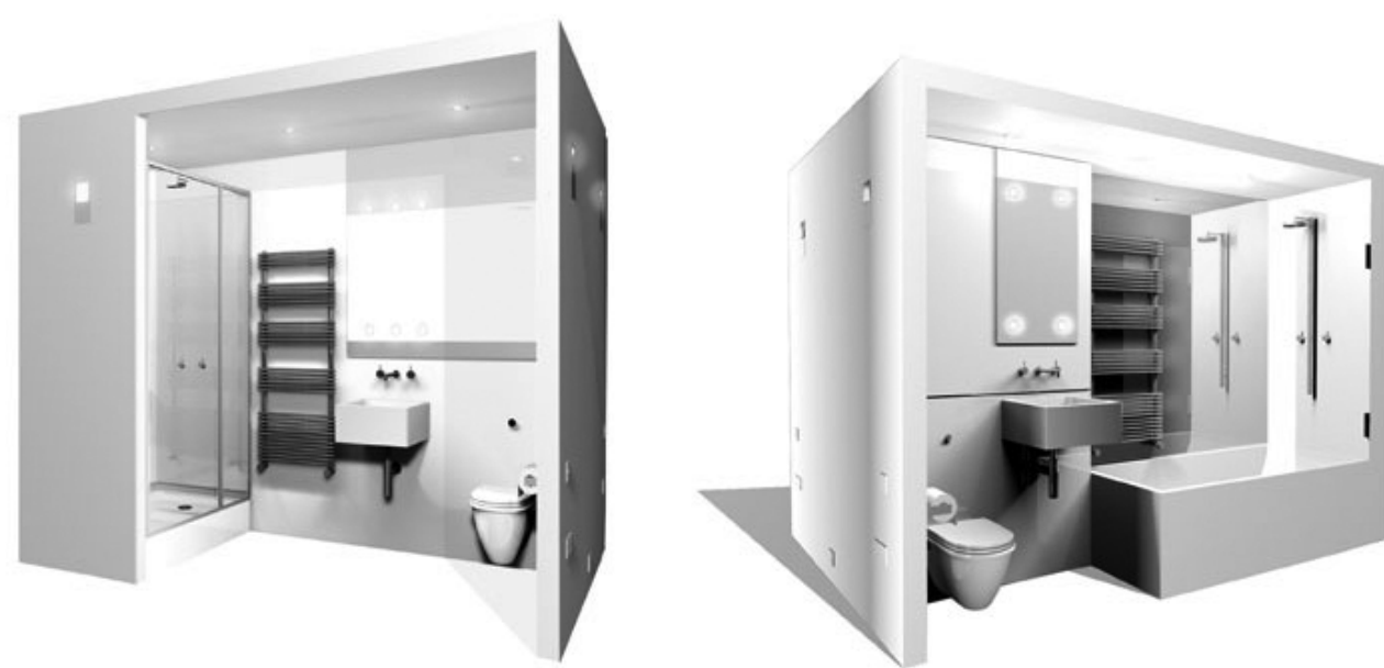
Centralized bathroom/kitchen cores avoid creating spatial interruption by means of avoiding unnecessary additional utilitarian chases.
