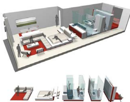
Creating a kit-of parts for the unit will create cohesion and ease of choice for the tenant.
